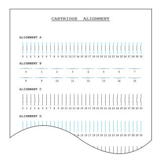
By selecting the straightest line for each pattern, you will optimise the print head alignment.
